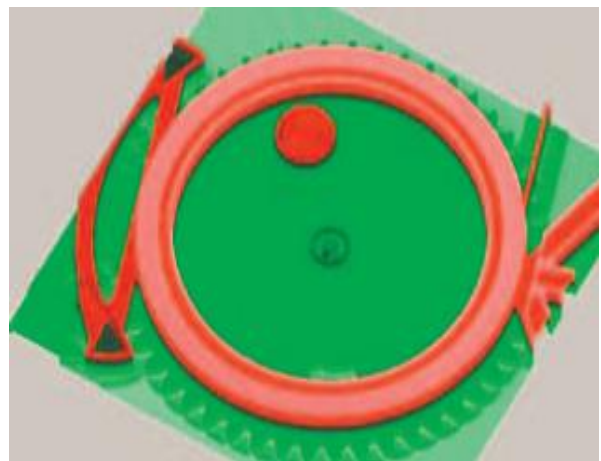
Figure 7: Topography measurement of a micro gearwheel
